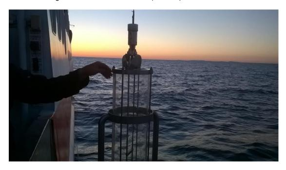
Figure 5. 30 L water sampler was used for monitoring of phycotoxins from different water layers (between 0-10m) and for microliter just below the clines. Photo: Maiju Lehtiniemi.
