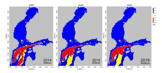
Figure 2. Oxygen conditions on the bottom in August 2014, 2015 and 2016. Blue indicates good oxygen conditions, yellow depleted oxygen and red anoxia.
