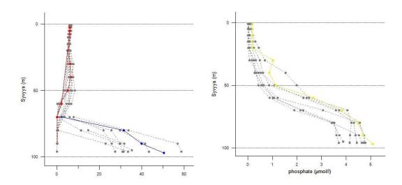
Figure 3. Oxygen and hydrogen sulfide profiles on the station F62 on the southwestern coast of the Gulf of Finland 2005-2016 (left). Profile of the present cruise is shown with red (oxygen) or blue (hydrogen sulfide) color. Depth (m) on y-axis, oxygen level (ml<sup>-1</sup>l) and hydrogen sulfide on the x-axis. Phosphate levels at the southwestern station F62 2008-2016 (right). Profile of the present cruise is shown with yellow color. Depth (m) on y-axis, phosphate level (µmol -1) on the x-axis.
